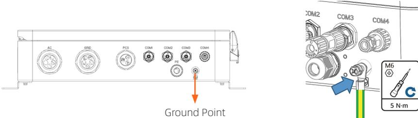
**⚠ CAUTION** Ensure that the ground cable is properly connected. If it is disconnected or loose, electric shocks may occur.
