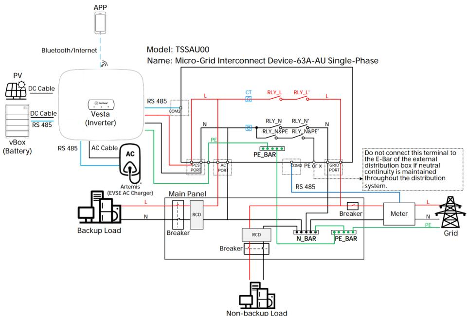
The diameter of the wire connected to the Main Panel and the N wire and PE wire in the Main Panel is 13.3 square millimeters, and the maximum current is 75A.
