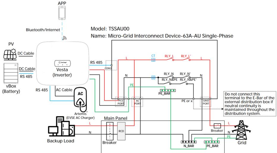
The diameter of the wire connected to the Main Panel and the N wire and PE wire in the Main Panel is 13.3 square millimeters, and the maximum current is 75A.
