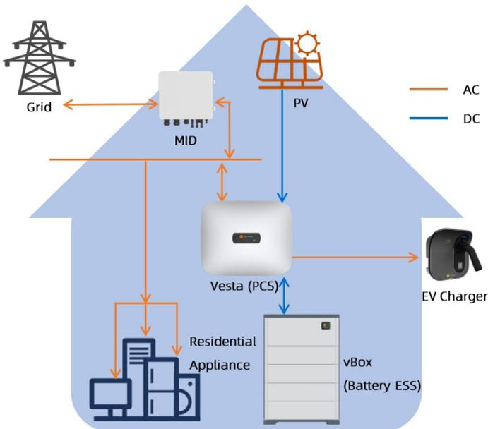
With Star Charge, we offer the complete system solution, including ESS vBox, Vesta inverter, EV charger, and MID device. With these components we can establish a complete residential PV, storage, and EV charger system. The key features of this system are managing PV, Storage & Charger output/input with a single AC device. The benefits are as follows:
